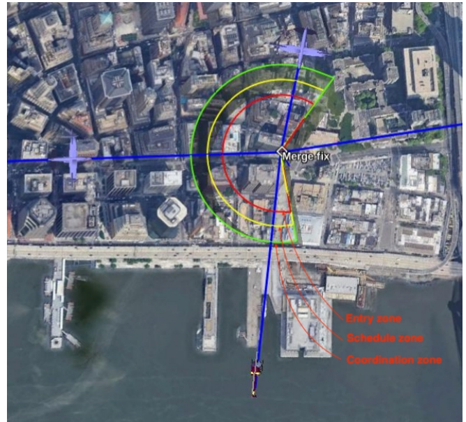
Fig. 2. A merge fix located in an urban environment. Various zones are indicated by the concentric rings
