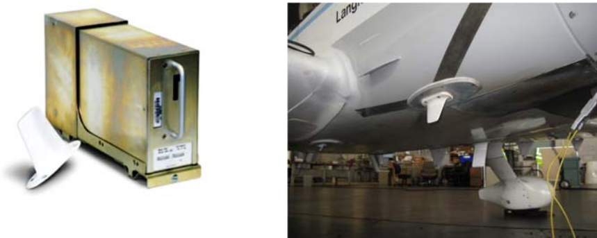
Figure 10 - Left: Garmin GDL 90 UAT. Right: UAT antenna mounted on bottom of Cirrus SR-22
