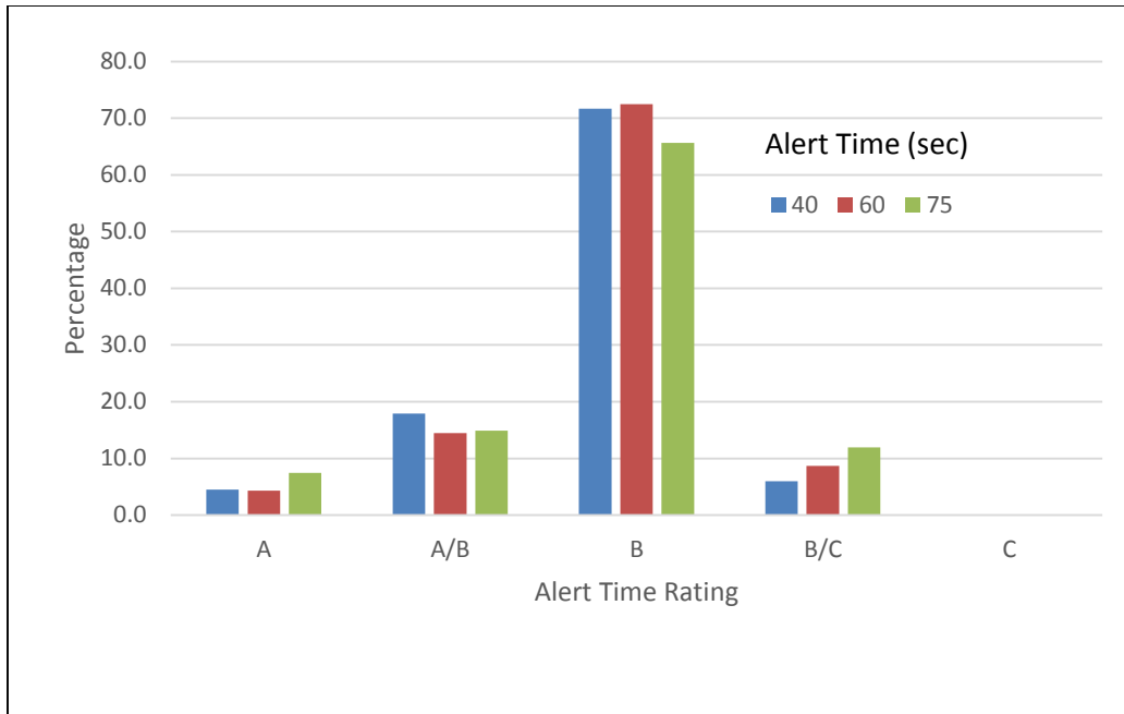
Figure 12. UAS Pilot ratings for Crossing Geometry Encounters with Alert Times of 40, 60, and 75 seconds (A = Too Early, B = Timing Okay, C = Too Late).
