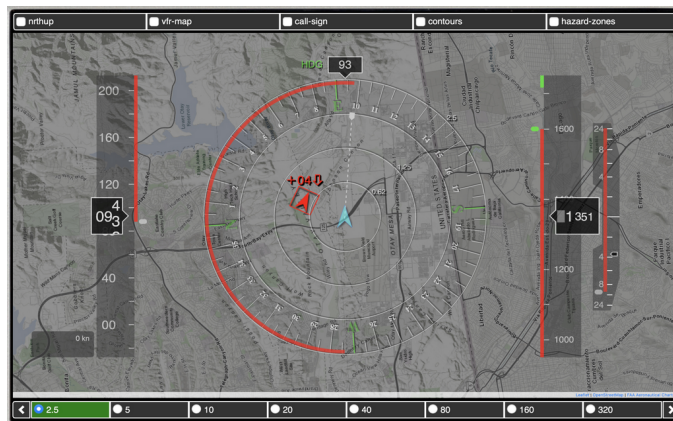
Fig 3. DANTi display, current trajectory in conflict
