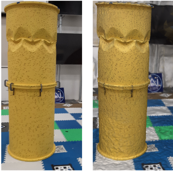
Fig. 12. Speckled Painting (left) and 3D Reconstruction (right)
