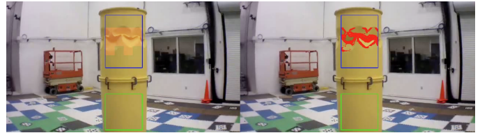
Fig. 11. CV Output of Segmented Satellites with Damage Highlighting
