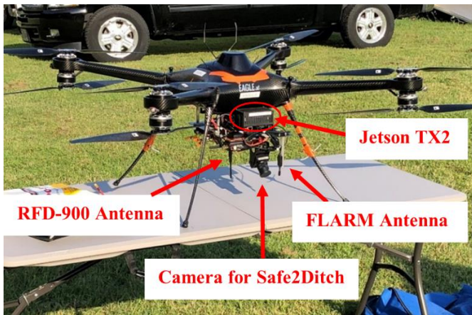
Fig. 2. UAVAmerica Eagle Octocopter used as alternate test vehicle
