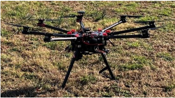
Fig. 1. DJI S-1000 Octocopter used as ownship and intruder vehicle
