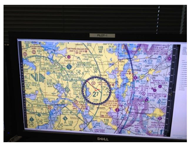
Figure 5. CAS-1 Moving Map Display for UAS and Manned Aircraft Pilots
