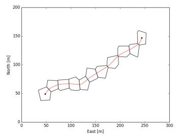
Figure 2: High-level path and corresponding flight plan
